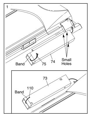
Insert the Right Upright (74) into the indicated bracket on the Base (83); be careful not to dislodge the Cage Nuts (76 [see the inset drawing]) from the Right Upright; in addition, be careful not to pinch the Upright Wire Harness (75). Finger tighten three Upright Bolts (72) with three Washers (78) and three Upright Star Washers (71) into the bracket and the Right Upright. Do not tighten the Upright Upright Bolts yet.
